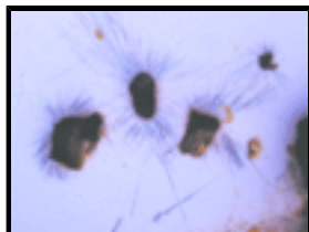
Fig. 2. Crystals of the title compound are the clear needles growing from the decomposed crystals of the lithium enolate.
